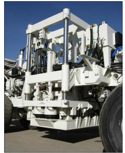
The Desert Explorer DX80 Actuator produces a force of 80,000 lbs.
