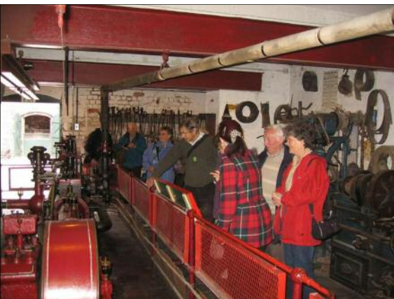
This is the steam engine which drives all the works at Gladstone, by belts and pulleys John Morgan
